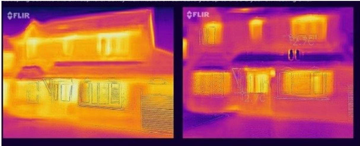
*BEFORE AND AFTER: Photo of the outside of a house taken by the thermal imaging camera showing before and after the fitting of cavity wall insulation.*
